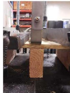
Photo 8: Typical Failure - Contact with Plywood
