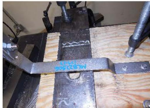
Photo 2: Tensile Test Setup
