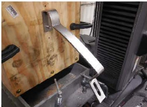
Photo 11: Deformation of Hook at Base
