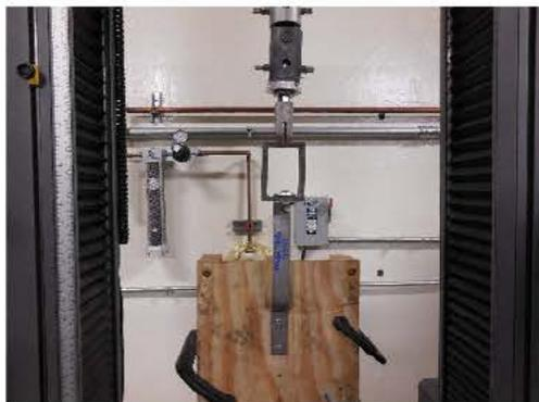
Photo 9: Shear Test Setup
